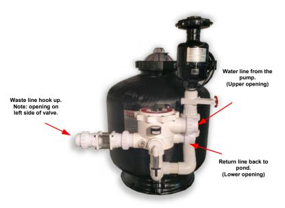
Make plumbing hook ups as shown in the picture. Use 2" pipe to connect to unions to secure plumbing to valve.
